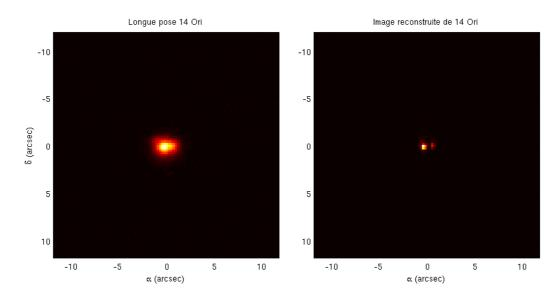
Image reconstruction test of the binary star system 14 Ori (H=4.6 magnitude), recorded in the astronomical H band (1.625 $\mu$ m) on October, 24 2014 at the Cassegrain focus of the 1 meter Omicron telescope of the C2PU facility (Observatoire de la Côte d'Azur). (left) Stack of 3000 co-added, 15ms exposure frames. (right) Reconstructed object from the 3000 short-exposure images.
