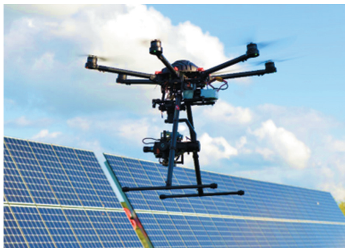
Figure 1: Drone with Raptor 640 SWIR camera
